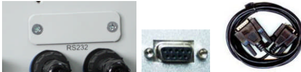
Fig. 10 RS232 serial port and special RS232 cable
